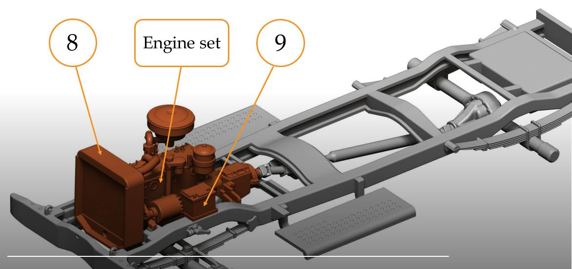
Engine, battery, cooler.
