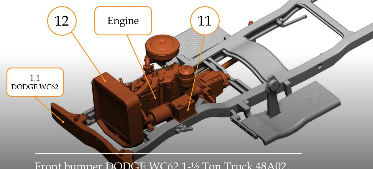
Front bumper DODGE WC62 1-½ Ton Truck 48A02, engine, radiator, battery
