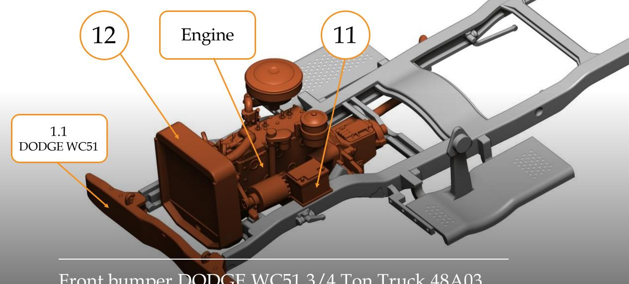
Front bumper DODGE WC51 3/4 Ton Truck 48A03, engine, radiator, battery
